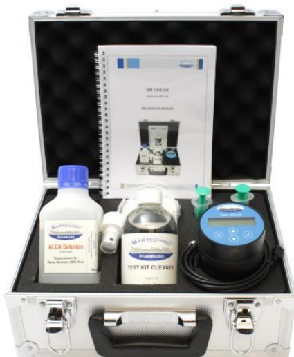
Test Kit „BN CHECK“ incl. Reagents and Accessories for Regular BN Measurements
